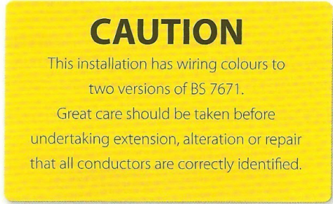
▼ Figure 6.12 Label advising of wiring colours to two versions of BS 7671
