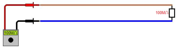
If the two final circuits are connected together in parallel, as they would be in a consumer unit/distribution board, their combined insulation will be less than that for one circuit; in this case  $50M\Omega$ .
